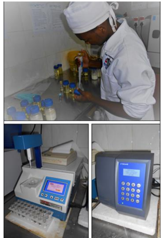
Figure 10. Micro analysis and equipment to analyse Freezing Point and SCC
