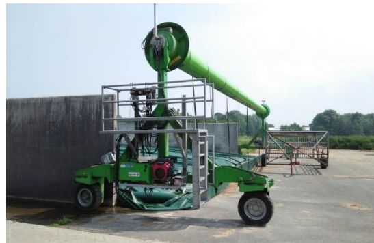
Picture 23: Movable Silage Covering Machine
