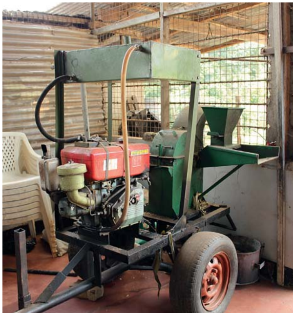
Equipment for chopping maize for silage on leased land.
