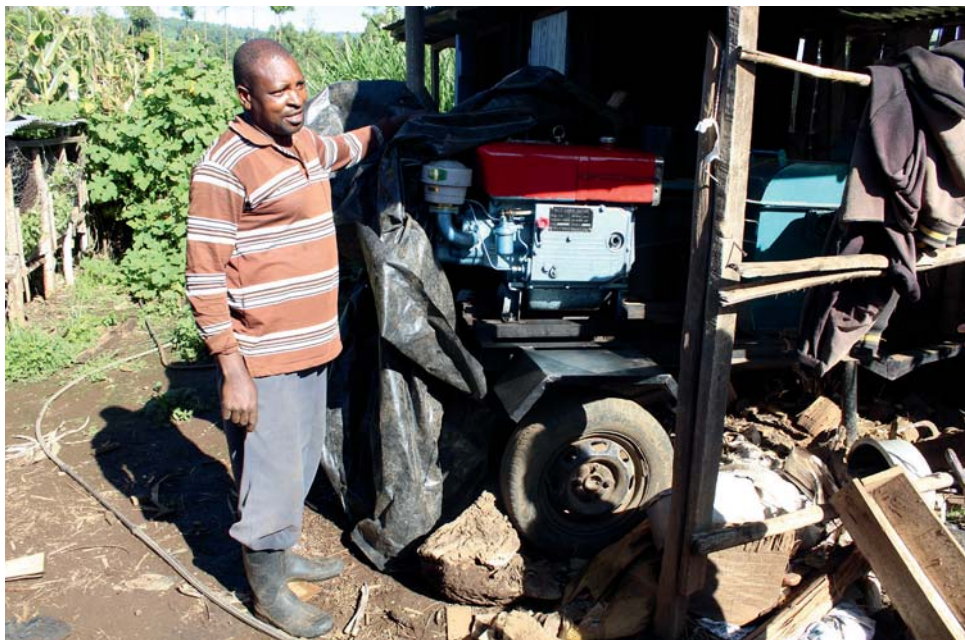
The diesel-powered chopping machine helps to break down the yellow maize for silage.
