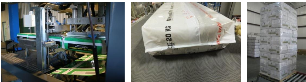
Figure 5.3 Baling and wrapping machine for 20-25 kg packs
