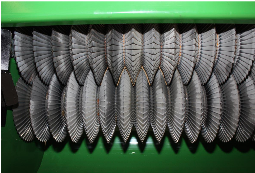
Figure 7. Example of a kernel processor on a modern harvester.
